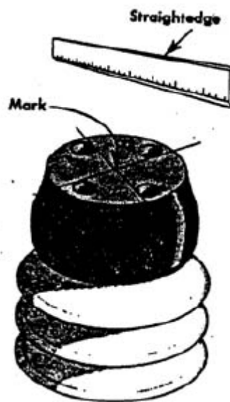
Figure 5: Find and mark exact center of rotating insulator.
